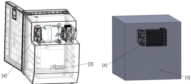
[3] 0,27in (Ø7mm) through-hole from the outside to the inside the cabinet to insert the temperature sensor.
