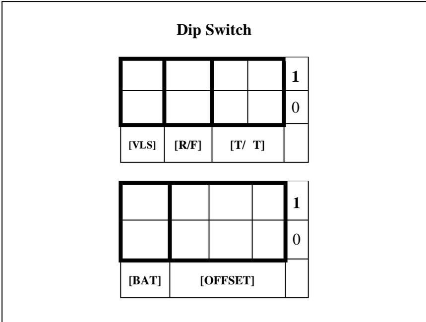
[OFFSET] compensates for the difference in temperature detected by the sensor and the actual temperature inside the cabinet.
