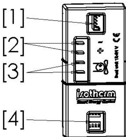
[1]: connection for the cable communicating the temperature data and controlling the potentiometer temperature.
