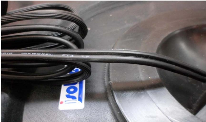
Whether the water-kit is 115V or 230V one of the pump wiring has writings on it. This wiring has to be connected on «L» while the other one on «N».
