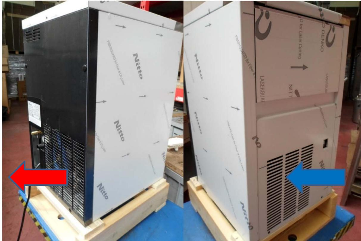
The ice-maker gets fresh air off the front grid and blows it out off the back
