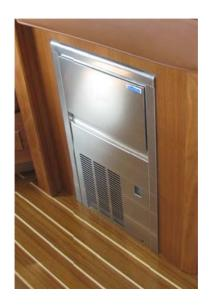
The Isotherm Clear Ice is stored in an insulated bin. The ice is always a "loose ice" meaning it never freezes into a clump like conventional 'white ice' makers. Because it is not stored in a freezer environment, the ice is always ready to be scooped out and is always slowly melting. Because of this, a drain hose must be connected and directed down to assure proper drainage.
