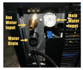
A drain hose (supplied with the unit) is connected to the water drain fitting. Since the ice is held in an insulated bin and not a freezer environment, it will always be slowly melting. The drain hose must be positioned to flow down for proper drainage.
